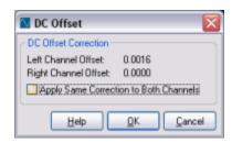
This feature lets you correct a DC offset in a sound file. A DC Offset is where the entire wave is shifted up or down, where zero is not quite zero. Some inexpensive sound cards may record audio with an offset that isn't quite zero; this feature will let you correct this.
